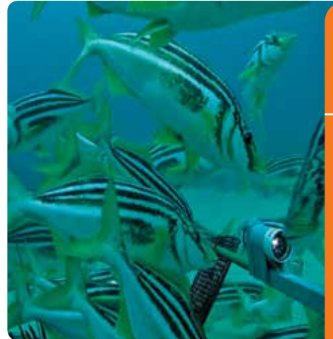
ABOVE LEFT: Photographic inventories of deep-water fish communities at 500 m depth were made for the first time in the Flinders CMR using Deep BRUVs: baited, instrumented, camera systems deployed on the seabed. Electronic controls initiate and synchronise the cameras, lights and bait delivery, enabling images to be collected for extended periods (weeks to months). Sensors measure environmental conditions.
