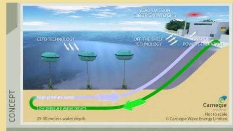
Wave-driven pumps Pipelines deliver high pressure water ashore Oriving proven hydroelectric generators
