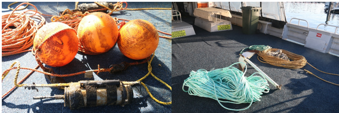
Figure 6 Photos of the vertical array. Left: The float system and SoundTrap used as an acoustic receiver. Right: The tethered system of rope and anchor used for the mooring.
