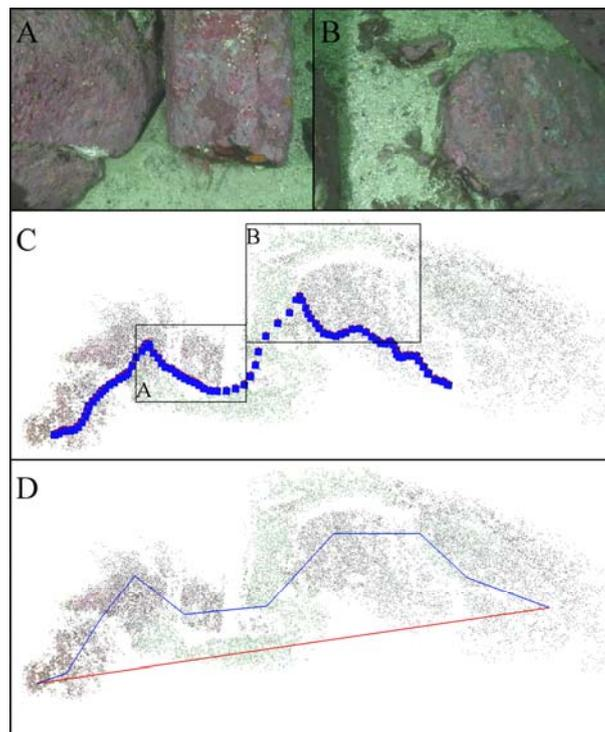
**Figure 1:** 3-D model of a sub-transect. (A, B) Two of the frames used to build the model (C) 3-D point cloud and reconstructed camera positions (blue squares) with the rough position of frames A and B. (D) 3-D points cloud, linear sub-transect length (red line) and projected sub-transect length (blue line).
