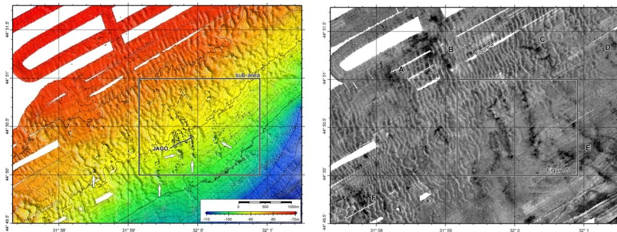
The left figure shows the bathymetric map of the study area, with white arrows indicating pockmarks and small black dots indicating gas release sites (vents). The right figure shows the backscattering of the multibeam with irregularly shaped discrete high backscatter patches (black) that match very nicely with the occurrence of bubble release (tiny white dots).
