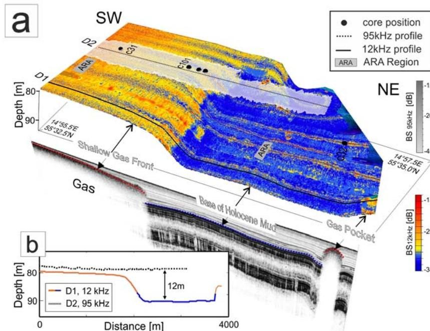
(a) Backscatter chart of EM120 (12 kHz, colored) and 95 kHz (grey, transparent) both draped onto their respective bathymetric grids. Strong variations in backscatter and bathymetry occur in the 12 kHz data with high backscattering strength values (BS) to the left (red, gas) and low ones (blue, no gas) to the right part of the figure. This corresponds to the underlying subbottom findings visible in the vertical
