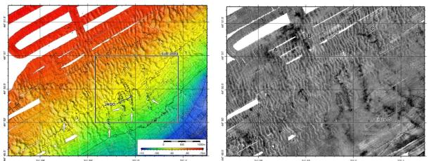
The left figure shows the bathymetric map of the study area, with white arrows indicating pockmarks and small black dots indicating gas release sites (vents). The right figure shows the backscattering of the multibeam with irregularly shaped discreet high backscatter patches (black) that match very nicely with the occurrence of bubble release (tiny white dots).
