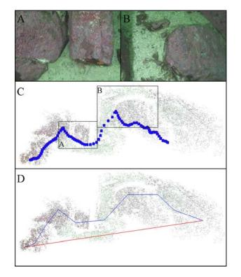
**Figure 1**: 3-D model of a sub-transect. (**A**, **B**) Two of the frames used to build the model (**C**) 3-D point cloud and reconstructed camera positions (blue squares) with the rough position of frames A and B. (**D**) 3-D points cloud, linear sub-transect length (red line) and projected sub-transect length (blue line).
