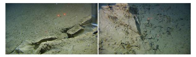
Seabed types at 2000 m water depth. Picture on the left shows foot of video-rig sinking into soft mud. Picture on the right shows compacted sediment block with gravel. Ten centimeters between red laser points.
