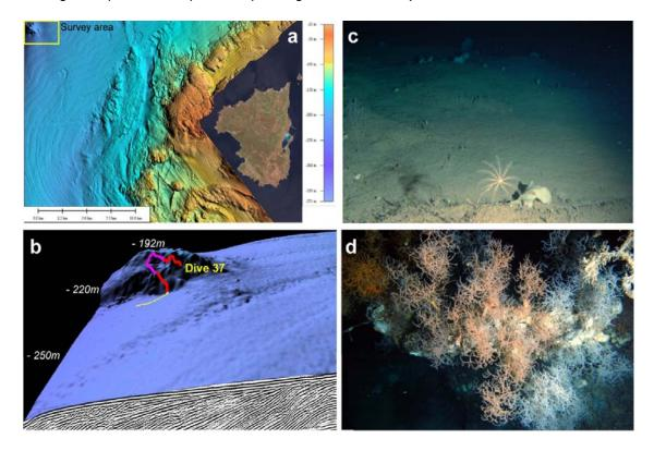
**Figures 1** - **a) Shadow relief from Multibeam** data of continental shelf offshore San Pietro Island, the Survey Area in the shelfbreak; (b) 3D display of DTM, showing the R. O. V course Dive 37, and the Sparker 500 J seismic section of the prograding late quaternary sequence; (c) Soft bottom (DL) with L.*phalangiu*m, *I.elongata* (d) Rocky bottom (RL) with *L.glaberrima*
