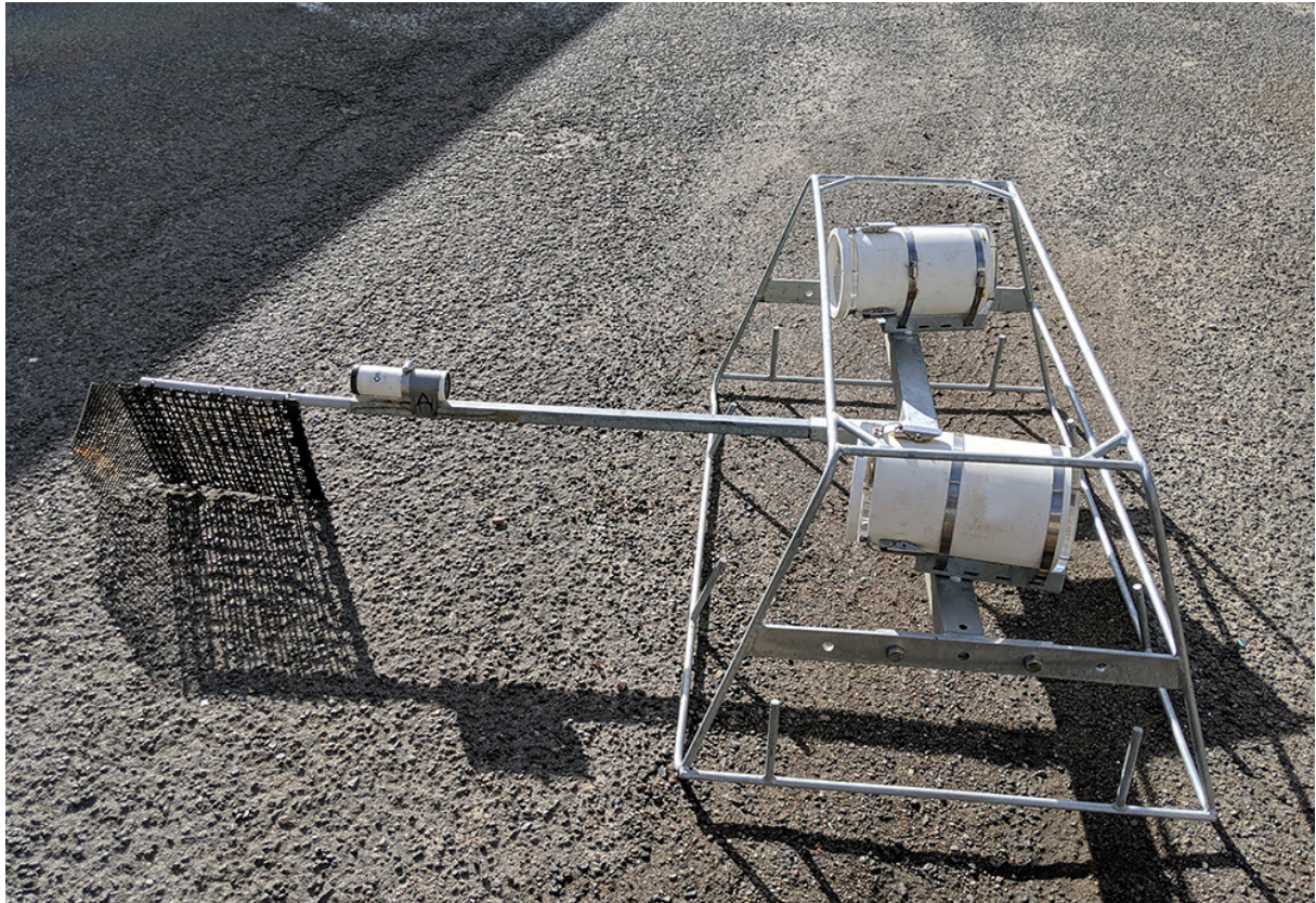
Figure 2: Photo of stereo-BRUVs system prior to deployment.
