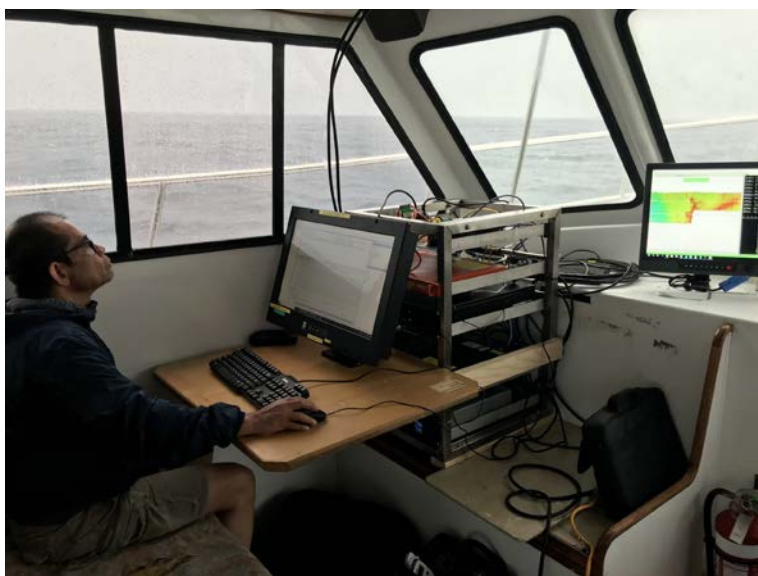
Figure 8. Multibeam sonar acquisition workstation on board FV Santosha
