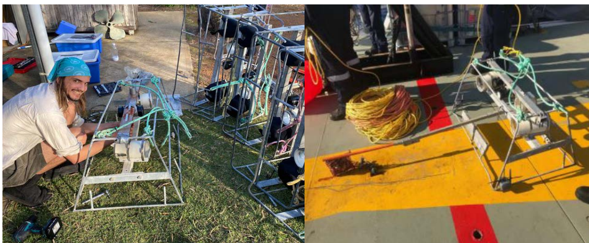
Figure 9. stereo-BRUV sampling equipment.
