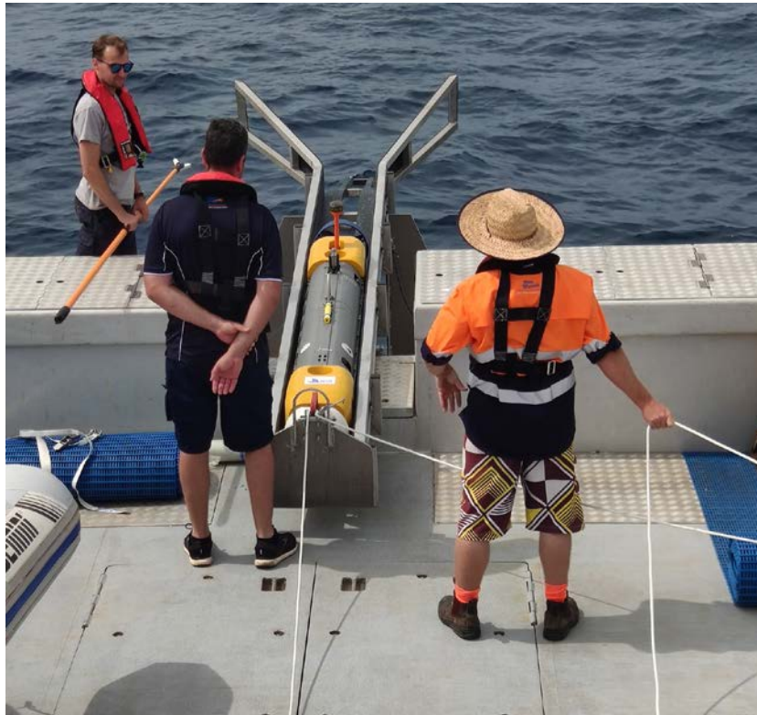
Figure 12. IMOS Autonomous Underwater Vehicle 'Nimbus'. AUV mounted on the launch and recovery system on the vessel.
