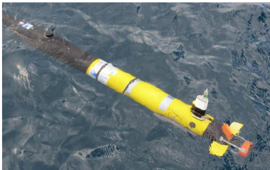
Figure 15 Photograph of the 'Iver' Autonomous Underwater Vehicle prior to diving to the seafloor (Photo credit: Kim Royce).
