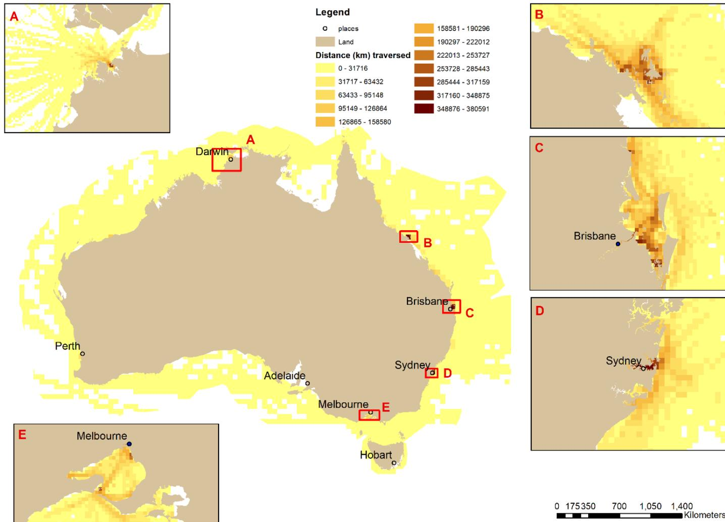
Figure 21 Distance traversed (km) per grid cell (1/2°) in 2015 for AIS equipped Recreational vessels, and example areas (1/30°) of higher density.
