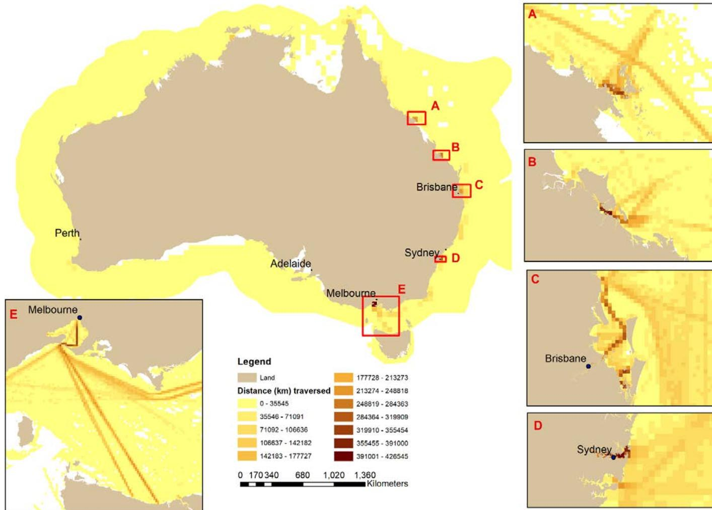
Figure 25 Distance traversed (km) per grid cell (1/2°) in 2015 for all AIS equipped vessels travelling faster than 15kts, and example areas (1/30°) of higher density. Note: Sydney harbour has speed restrictions except for ferries (as demonstrated by the high density in Figure 26)
