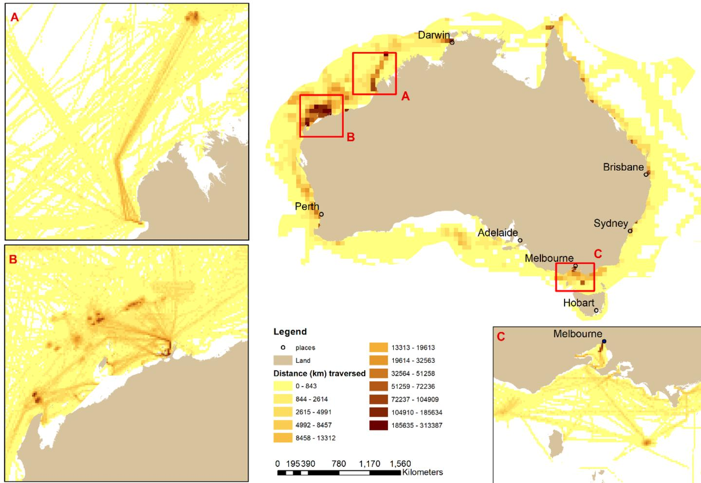
Figure 24 Distance traversed (km) per grid cell (1/2°) in 2015 for AIS equipped Working vessels (i.e., crew boats, offshore supply vessels, specialised vessels such as dredgers), and example areas (1/30°) of higher density.
