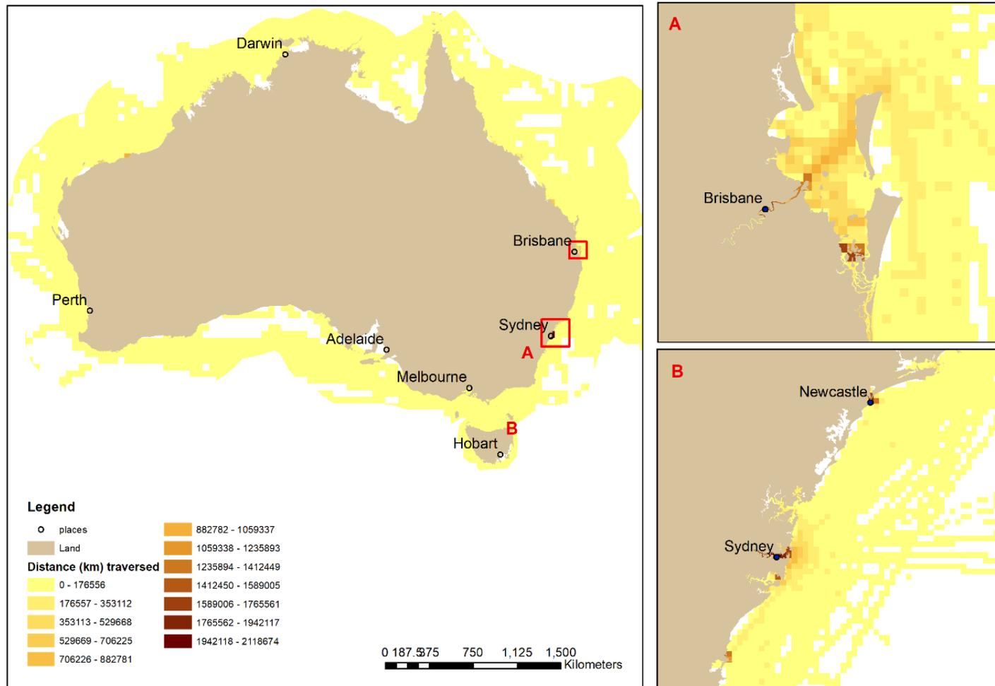
Figure 10 Distance traversed (km) per grid cell (1/2°) in 2015 for AIS equipped vessels with length between 25m - 50m, and example areas (1/30°) of higher density.
