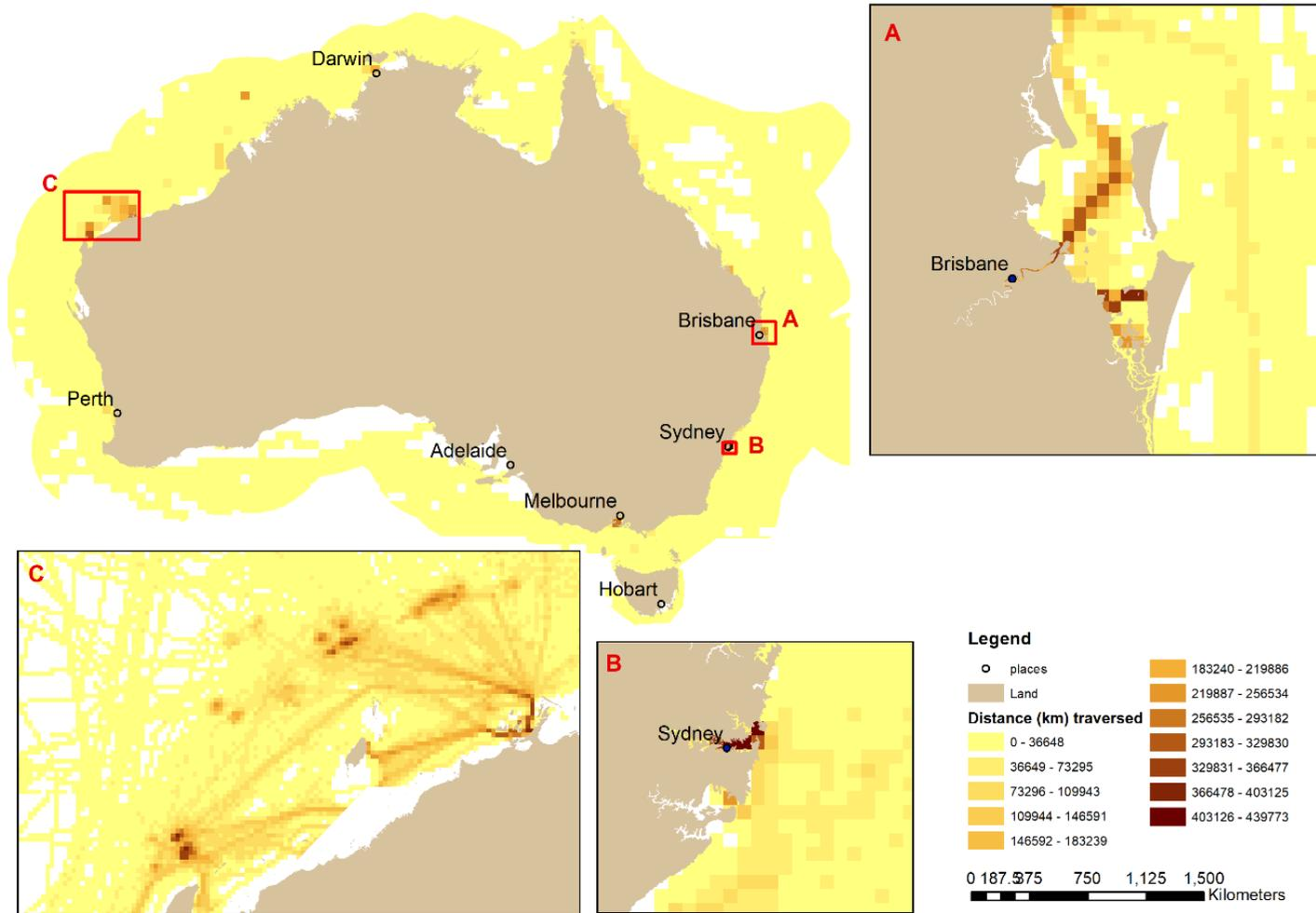
Figure 11 Distance traversed (km) per grid cell (1/2°) in 2015 for AIS equipped vessels with length between 50m - 100m, and example areas (1/30°) of higher density.
