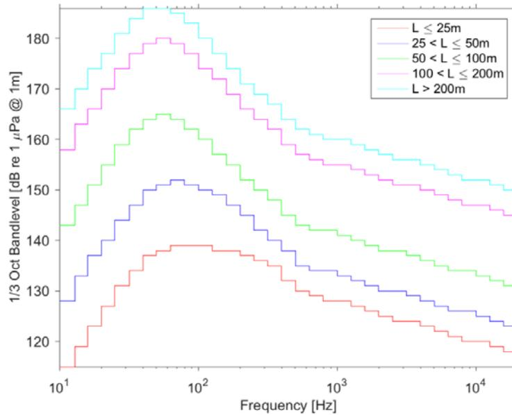
**Figure 85** Estimated source level spectra of ships recorded using the IMOS recorders for five size classes of vessel (n = 92 vessels)
