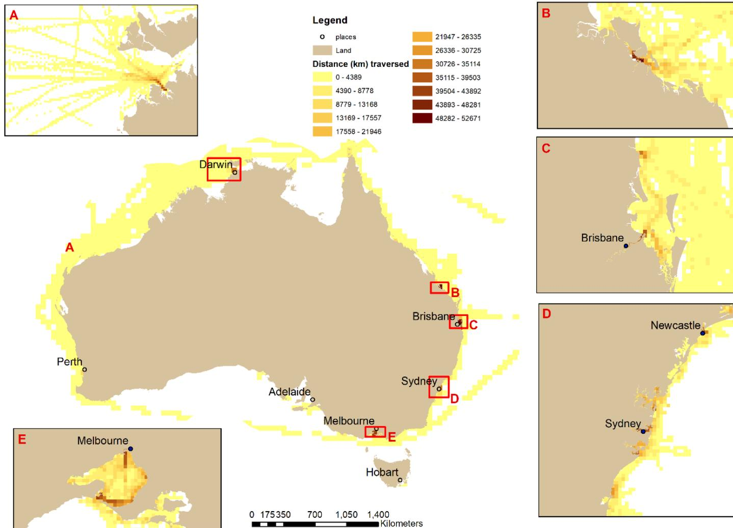
Figure 19 Distance traversed (km) per grid cell (1/2°) in 2015 for AIS equipped Official(i.e., Police, ranger, customs, search and rescue etc) vessels, and example areas (1/30°) of higher density.
