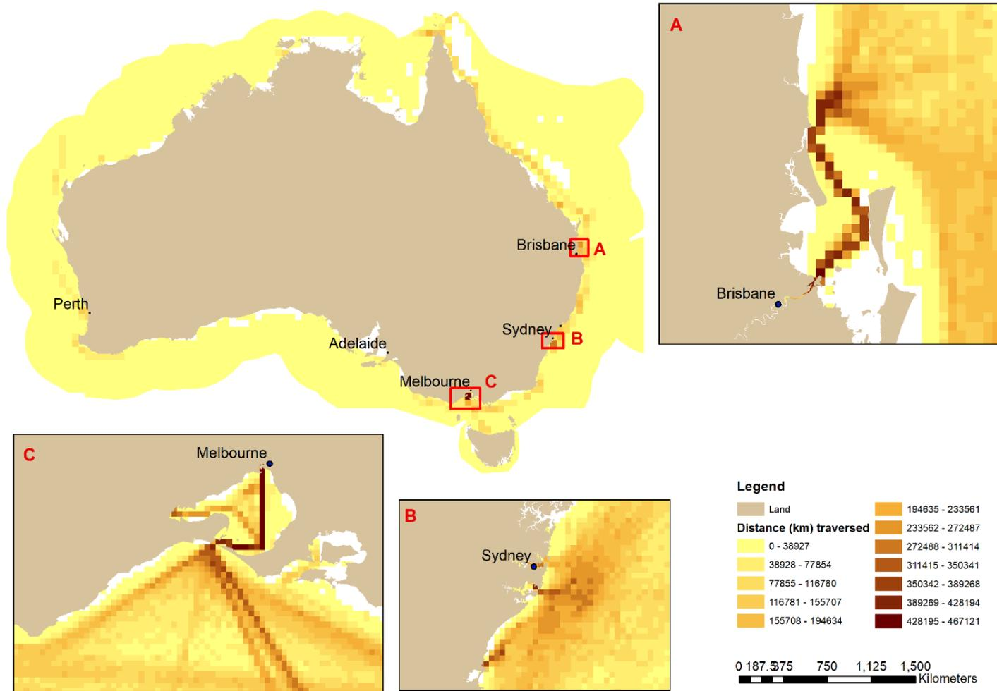
Figure 12 Distance traversed (km) per grid cell (1/2°) in 2015 for AIS equipped vessels with length between 100m-200m, and example areas (1/30°) of higher density.
