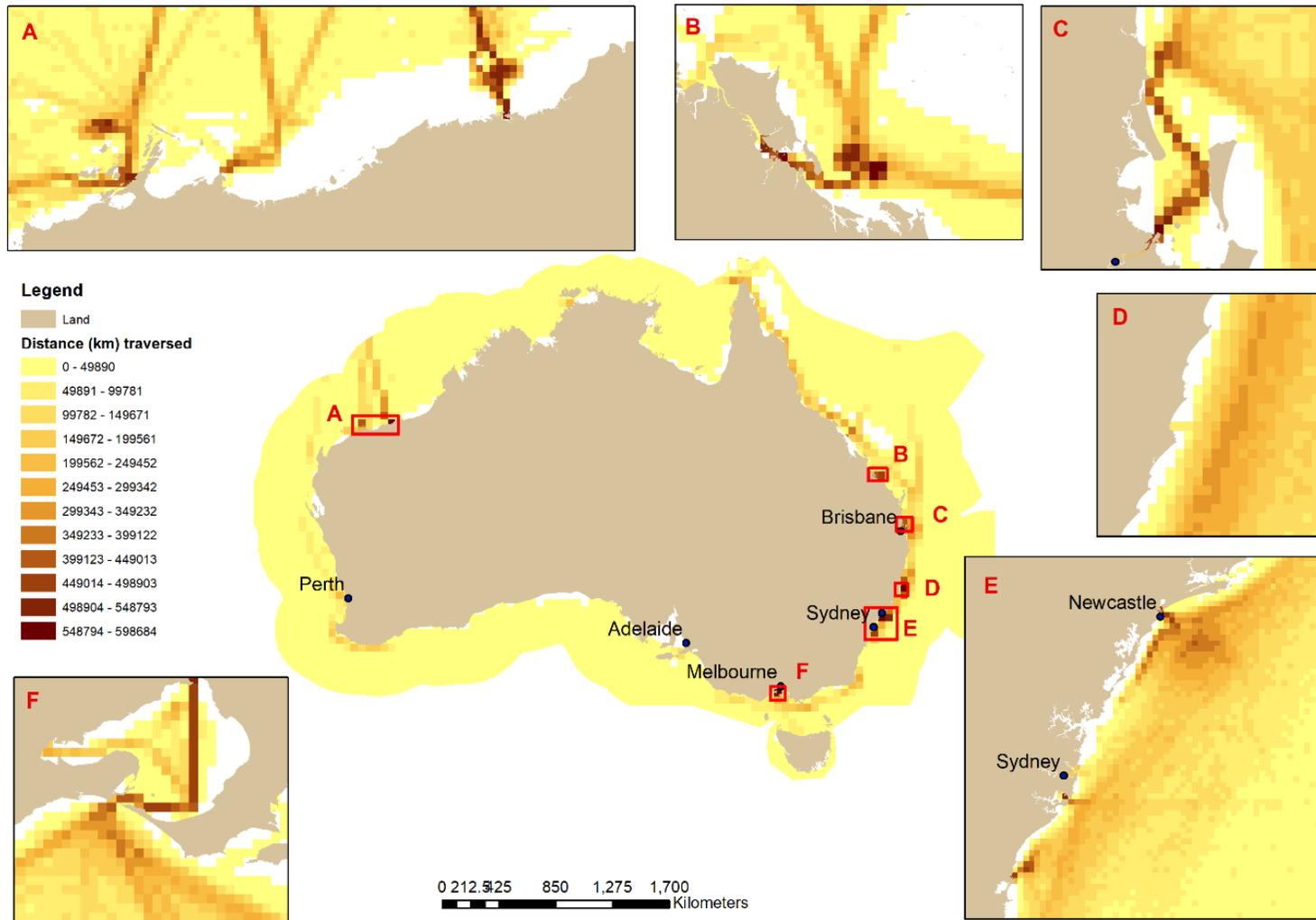
Figure 15 Distance traversed (km) per grid cell (1/2°) in 2015 for AIS equipped Cargo vessels, and example areas (1/30°) of higher density.
