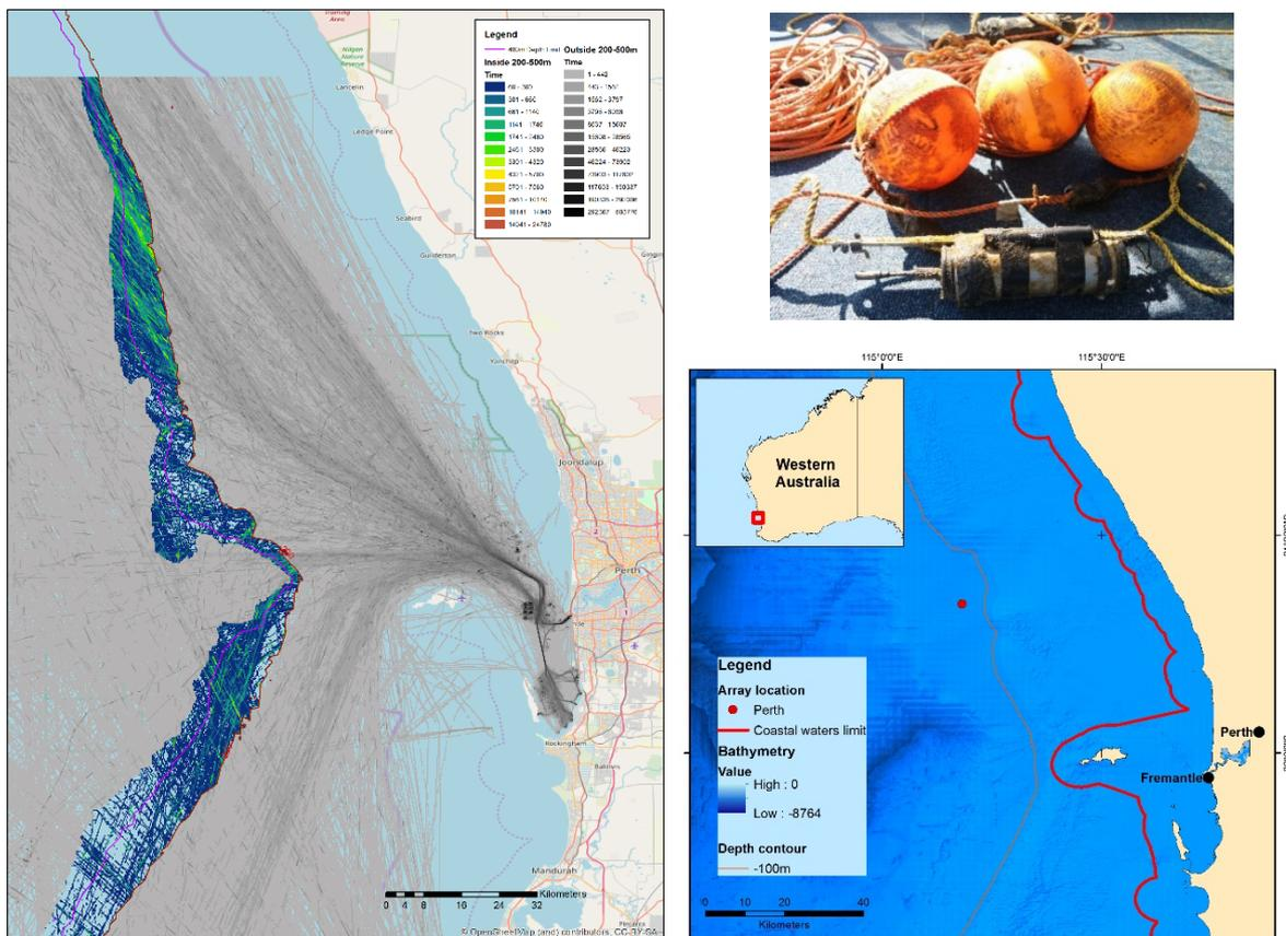
Figure 3 Mapping of AIS-equipped vessel traffic for determination of suitable logger deployment sites (left), 3D array (top right) and location of logger (bottom right)
