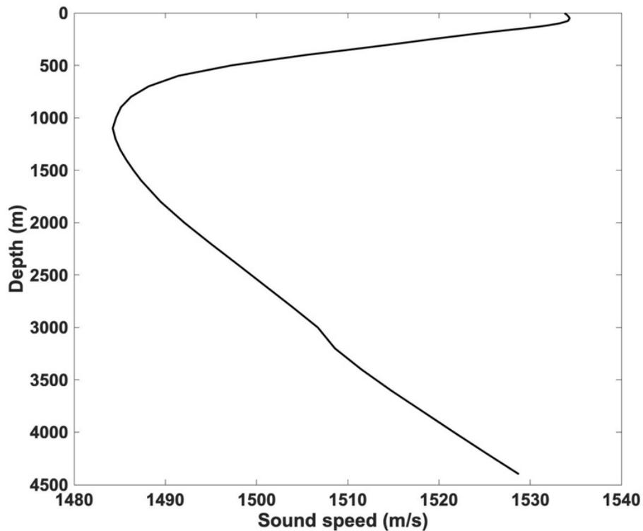
**Figure 23. Sound speed profile for the Great Barrier Reef ship noise propagation model**
