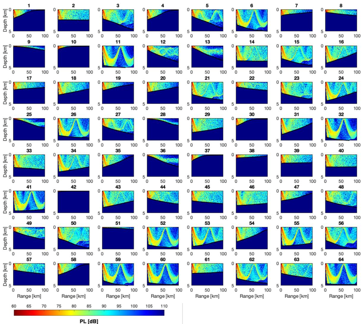
**Figure 12** Plots of propagation loss (PL) in dB as a function of range and depth along the 64 centroid bathymetries from Zone 15, for a frequency of 640 Hz. The darkest red corresponds to 60 dB and the darkest blue to 110 dB. X-axes are range [km] and Y-axes are depth below the sea surface [km], scaled linearly.
