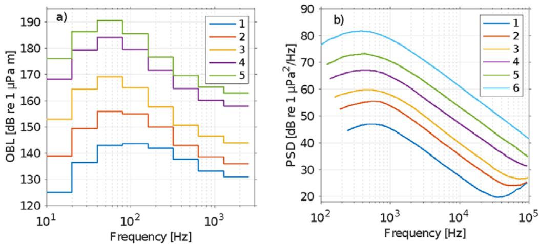
**Figure 14** a) Ship source levels as full-octave band levels (OBL) for ships of length classes <25 m (Class 1), ≥25 - <50 m (Class 2), ≥50 - <100 m (Class 3), ≥ 100 - <200 m (Class 4), and ≥200 m (Class 5). b) Power spectral density levels (PSD) of wind noise at wind speeds ≥1 - <3 kn (Curve 1), ≥3 - <7 kn (Curve 2), ≥7 - <11 kn (Curve 3), ≥11 - <21 kn (Curve 4), ≥21 - <48 kn (Curve 5), and ≥48 kn (Curve 6).
