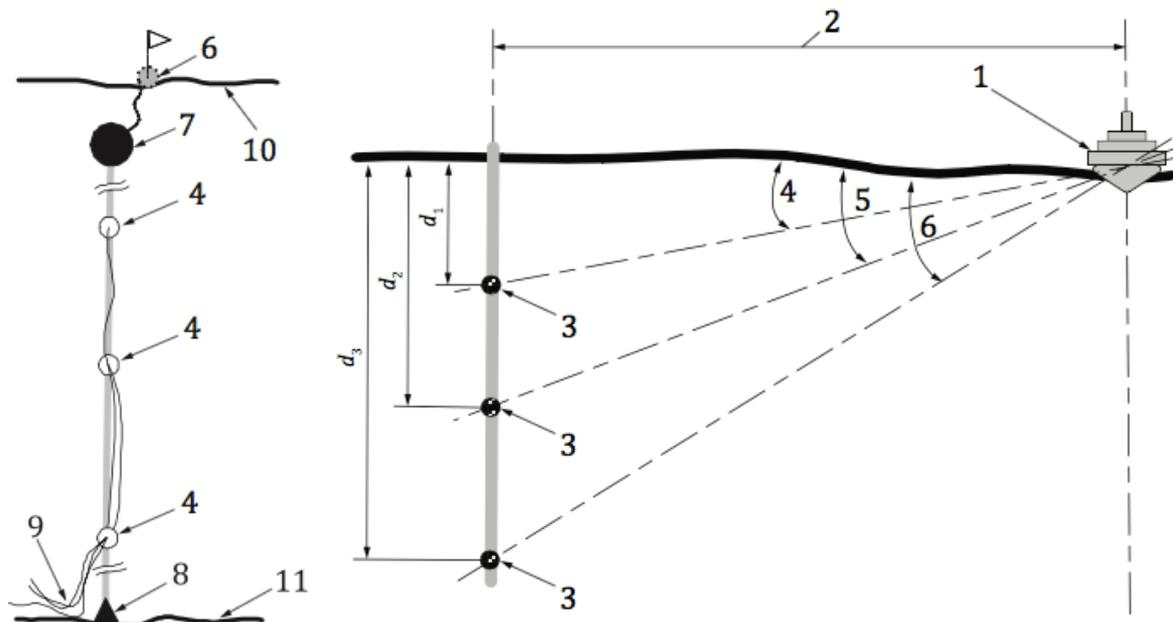
**Figure 2 Left: Sketch of a vertical array for ship noise measurements** It consists of the hydrophones (4), an optional surface buoy (6), a subsurface float (7), an anchor (8), signal lines to shore (9) unless autonomous recorders are used at the locations 4, sea surface (10) and seafloor (11). Right: Sketch of a ship (1) passing at distance (2) from the hydrophone array (3), whereby the hydrophones are at slant
