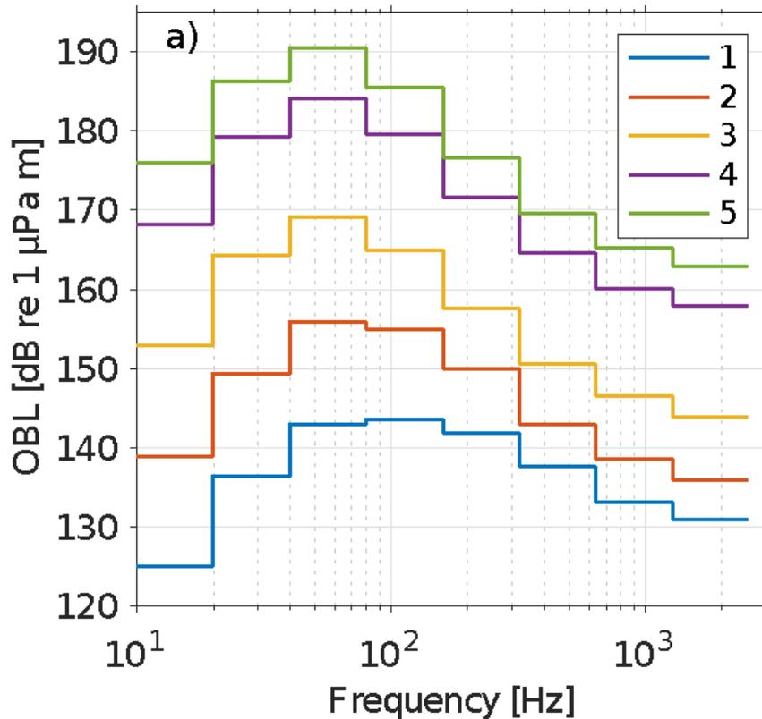
**Figure 4 Ship source levels as full-octave band levels (OBL) for ships of lengths <25 m (Class 1), ≥25 - <50 m (Class 2), ≥50 - <100 m (Class 3), ≥ 100 - <200 m (Class 4), and ≥200 m (Class 5)**
