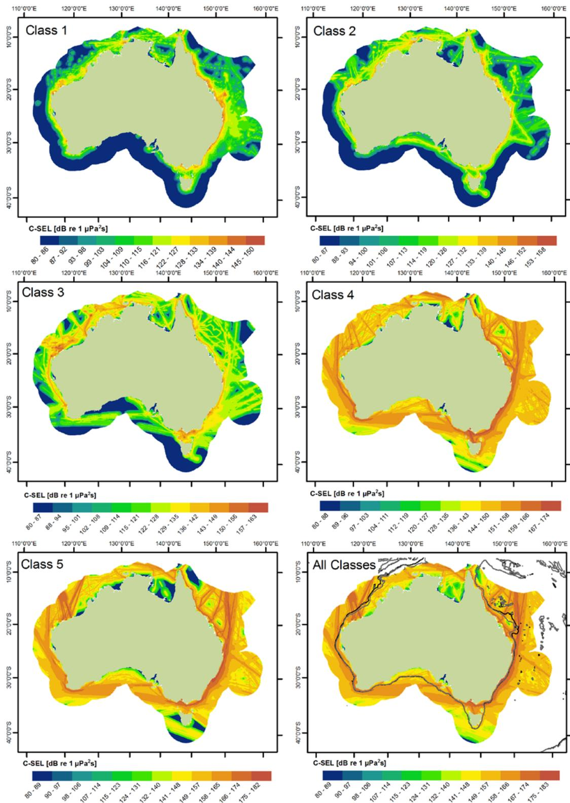
**Figure 13** Maps of cumulative sound exposure levels (C-SEL) from shipping in the Australian EEZ, by ship class, and cumulatively over all classes (Table 1).
