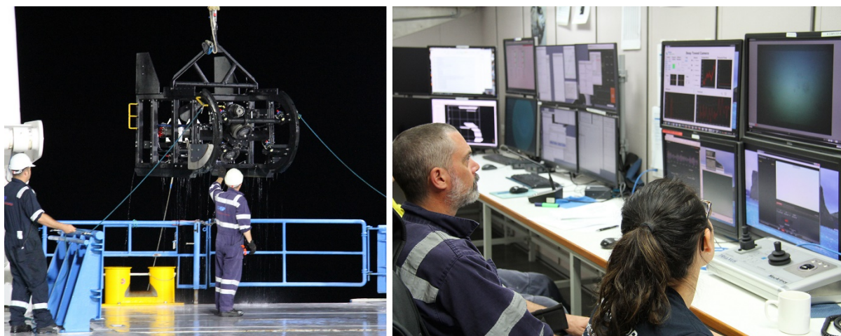
Figure 4 Towed video system (left) and operations room (right) of the R.V. Investigator during deployment
