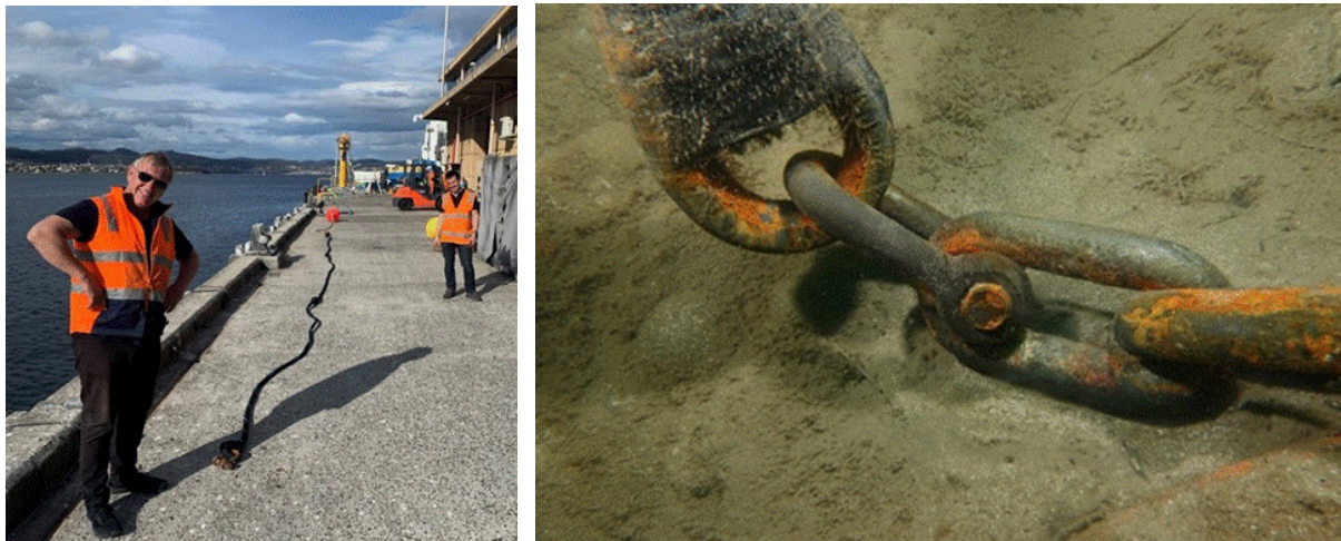
Figure 4-10 Rebuilt mooring for the Maple Leaf 42. Note the bulbous hardened node midway along the black strop. Mr Tim Fountain (CSIRO Mooring technician) is in the foreground and Mr Andrew Martini (CSIRO Engineer) is mid shot and b) attachment to the anchor and chain.
