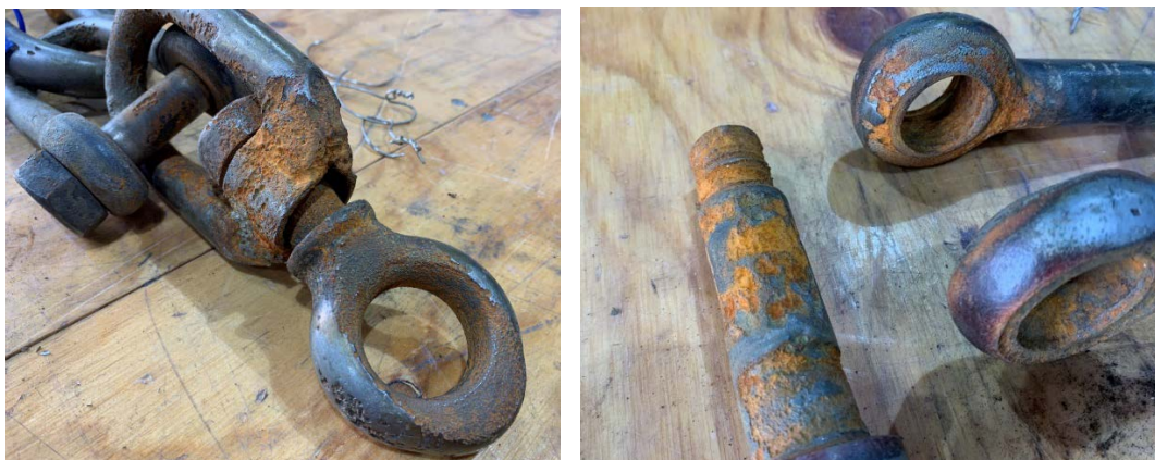
Figure 4-6 Severe corrosion from the Clansmann 30's hardware set
