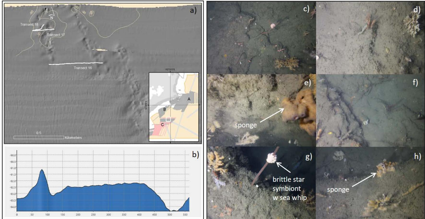
Figure 3-13. a) planar view of hill-shaded bathymetry with location of video transects (T16-18) offshore of Broughton Island (Area C) October 2019; b) bathymetric cross-section through transect (T16) start-end points; Transect 16 (c), 17 (d), 18 ((e-f) showing (c-h) erect sponges and corals, (c-h) sediment inundated reef with emergent sponges, (e, h) massive sponges, (g) sea whip with symbiotic brittle star (*Ophiruroidea*) and (h) sponges and bryozoans. Laser points are 100 mm apart.
