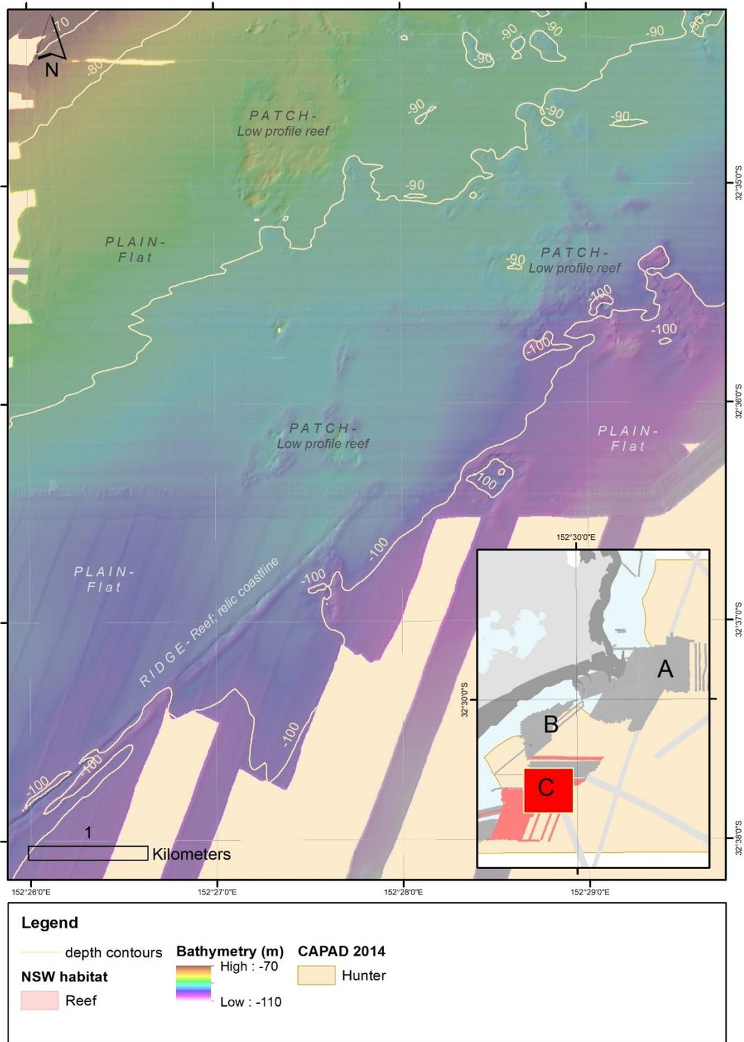
Figure 2-7. False-colour hill-shaded bathymetry of survey area C: Offshore Broughton and seabed features - northern section
