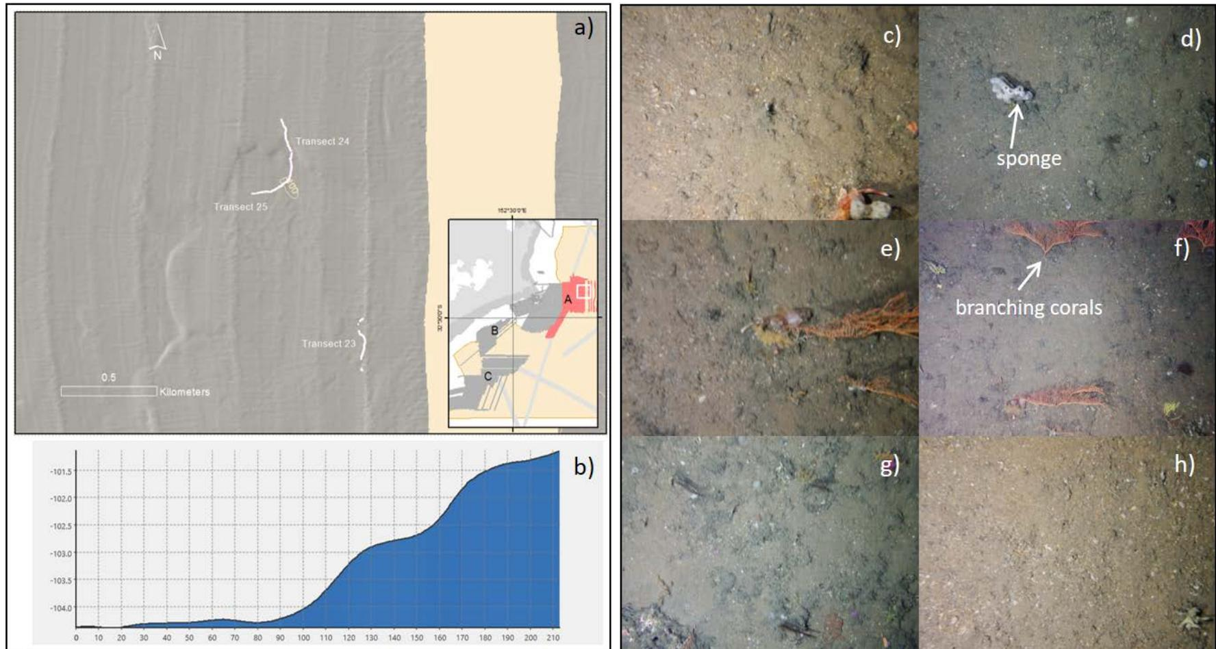
Figure 3-7. a) planar view of hill-shaded bathymetry with location of video transects (T24) at Seal Rocks (Area A) October 2019, (*nb. north-south oriented parallel ridges are MBES artefacts*); b) bathymetric cross-section through transect (T24) start-end points; Transect 24 imagery showing (c-g) veneered soft sediment and sponges, (e-f) corals, (c-d, g) sparse sponges and cobble rubble and (c, h) infaunal sediment burrows and rubble. Laser points are 100 mm apart.
