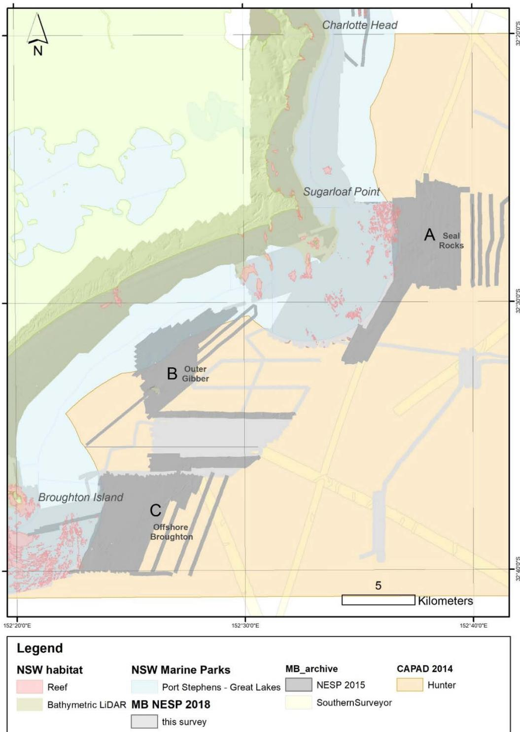
Figure 2-1. Extent of new survey areas (A - Seal Rocks; B - Outer Gibber; and C – Offshore Broughton), existing multibeam surveys, bathymetric LiDAR (LADS) and digitised rocky reef (NSW state waters) within the Special Purpose Zone of the Hunter Marine Park and adjacent Port Stephens - Great Lakes Marine Park areas.
