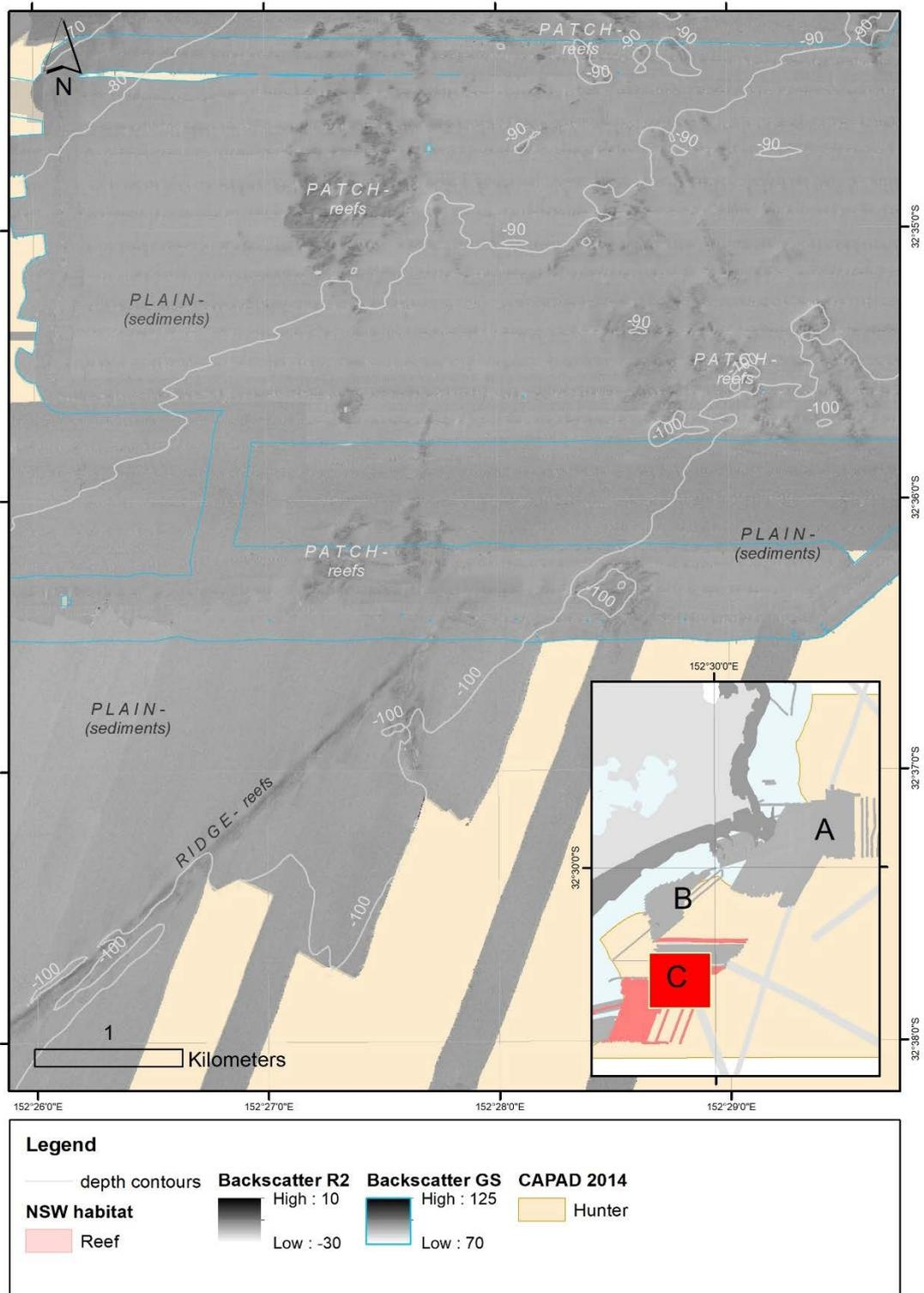
Figure 2-8. Grayscale backscatter (seabed reflectance) for survey area C: Offshore Broughton and seabed features - northern section
