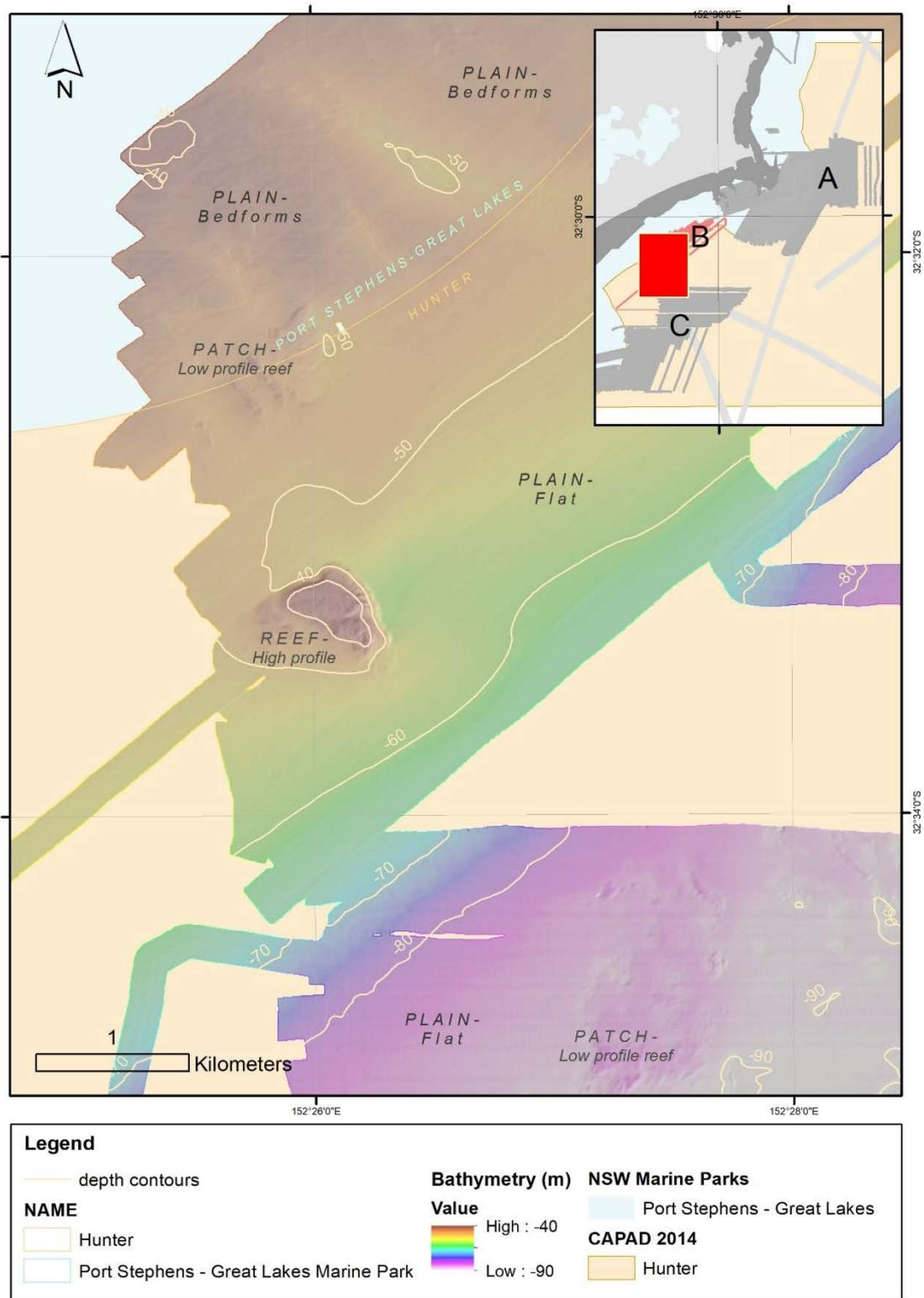
Figure 2-5. False-colour hill-shaded bathymetry of survey area B: Outer Gibber and seabed features
