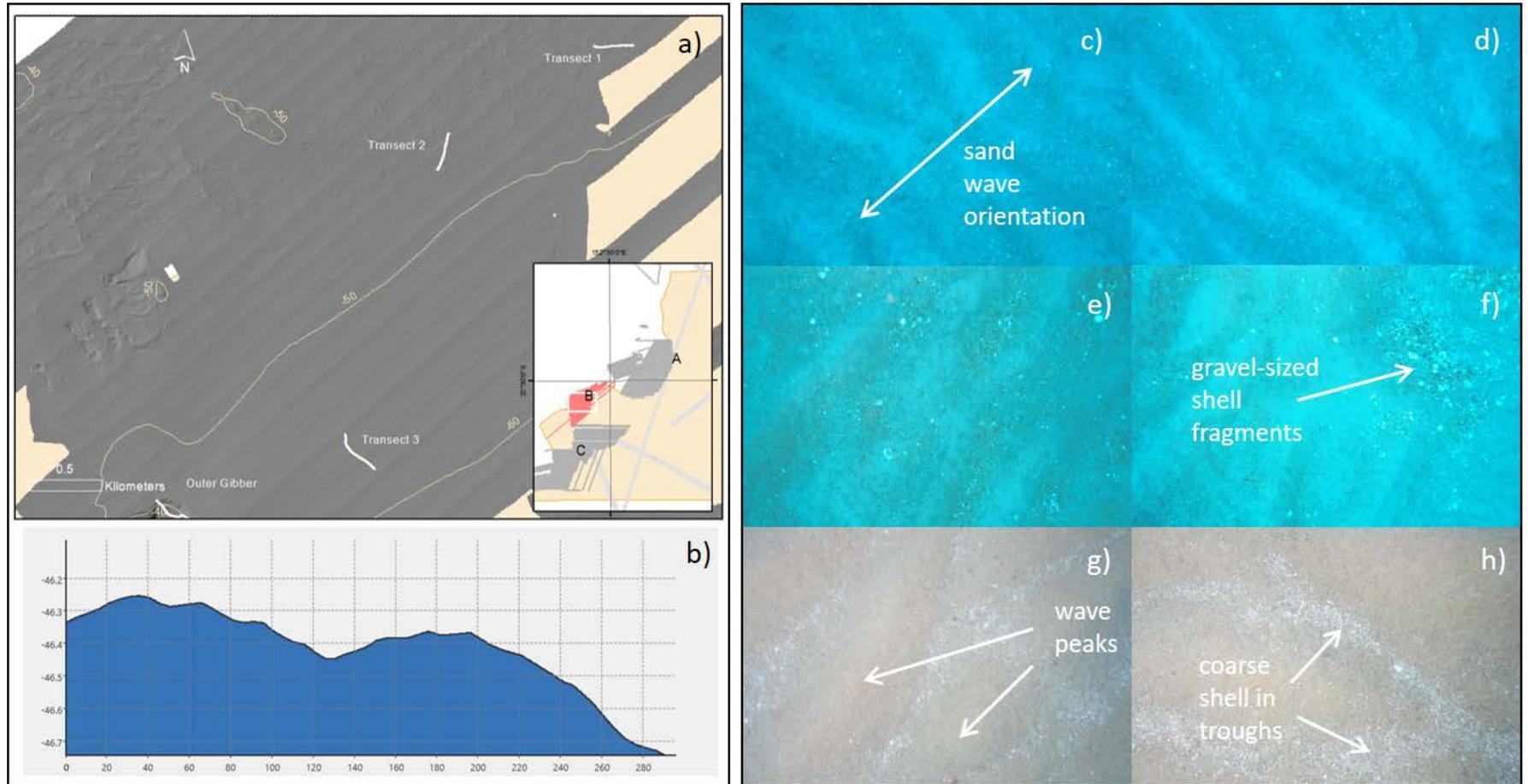
Figure 3-9. a) planar view of hill-shaded bathymetry with location of video transects (T1-3) north of Outer Gibber (Area B) October 2019; b) bathymetric cross-section through transect (T1) start-end points; Area B – Outer Gibber: Downward looking still imagery from along Transects 1 - 3 showing (c-h) soft sediment habitat with sand waves with coarser shelly material located in sand wave troughs. Laser points are 100 mm apart.
