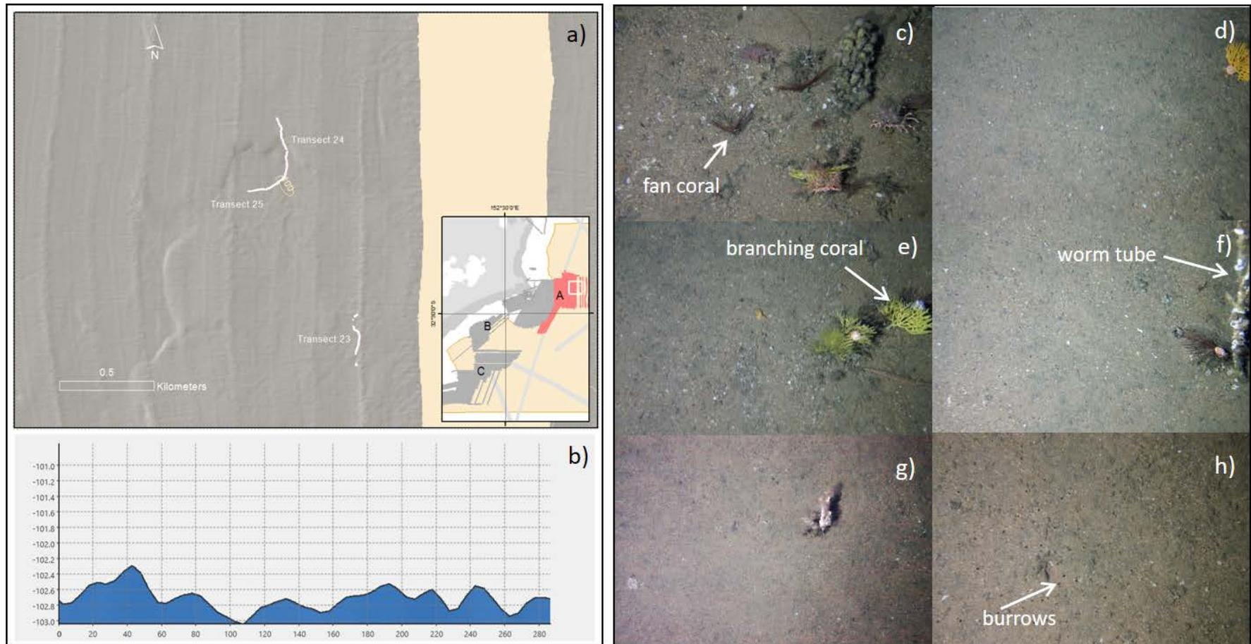
Figure 3-6. a) planar view of hill-shaded bathymetry with location of video transects (T23) at Seal Rocks (Area A) October 2019, (*nb. north-south oriented parallel ridges are MBES artefacts*); b) bathymetric cross-section through transect (T23) start-end points; Transect 23 imagery showing (c-g) small erect sponges, branching cnidarian fan corals, and worm tubes; and (g-h) soft sediment infaunal burrows. Laser points are 100 mm apart where visible.
