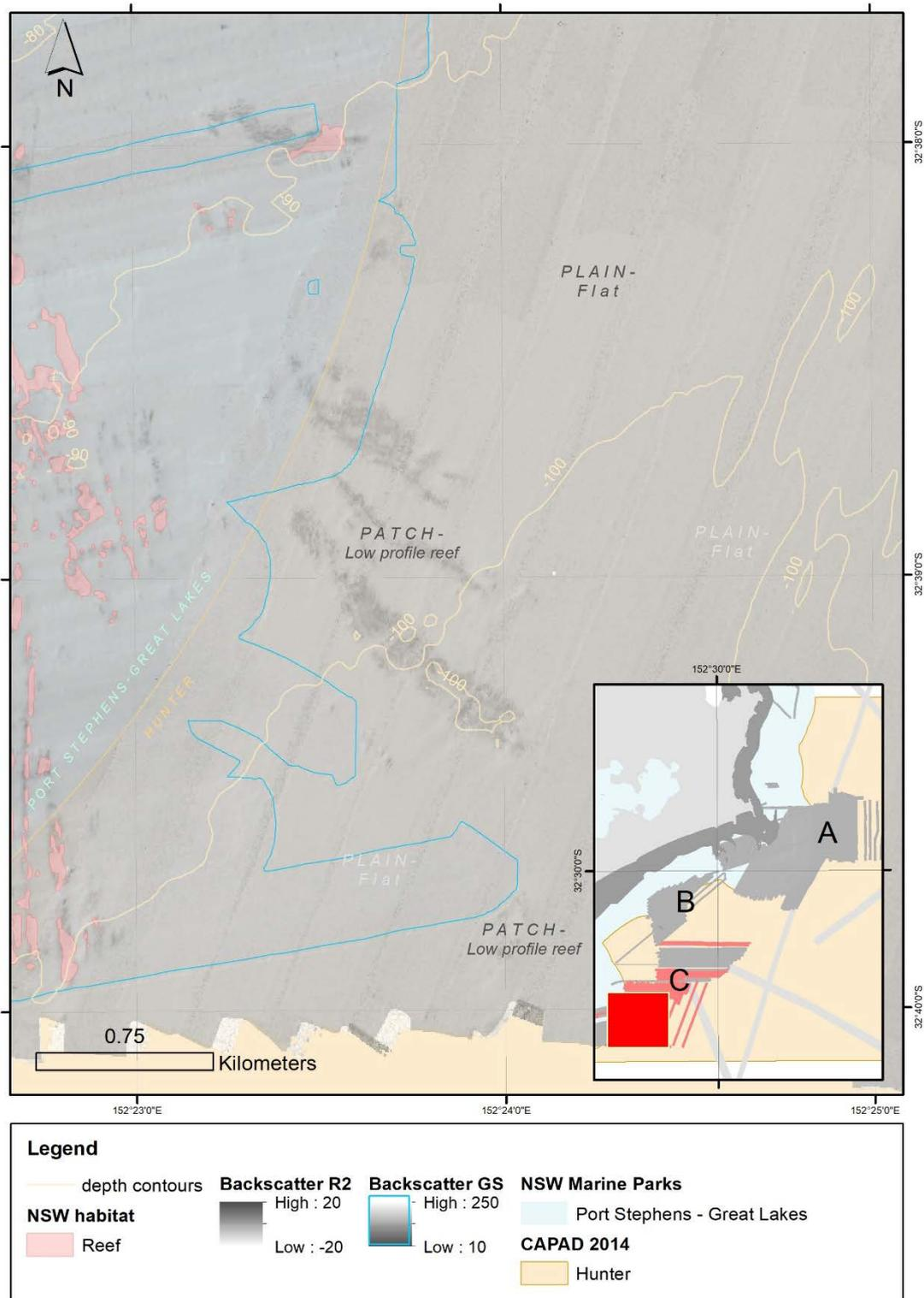
Figure 2-10. Greyscale backscatter (seabed reflectance) for survey area C: Offshore Broughton and seabed features - northern section
