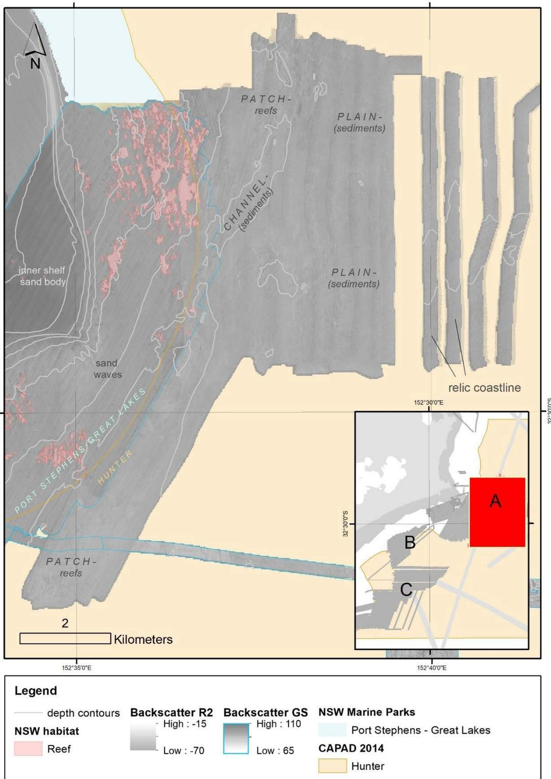
Figure 2-4. Greyscale backscatter (seabed reflectance) for survey area A: Seal Rocks and seabed features
