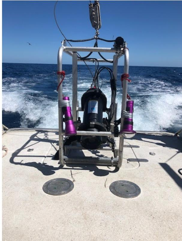
Figure 3-1. NSW DPIE Towed Video fish setup showing centred forward-looking video camera with live fish-to-surface fibre optic feed and lights, rear deck of RV Bombora (the digital stills camera sits toward the back of the tow-frame and not visible here).
