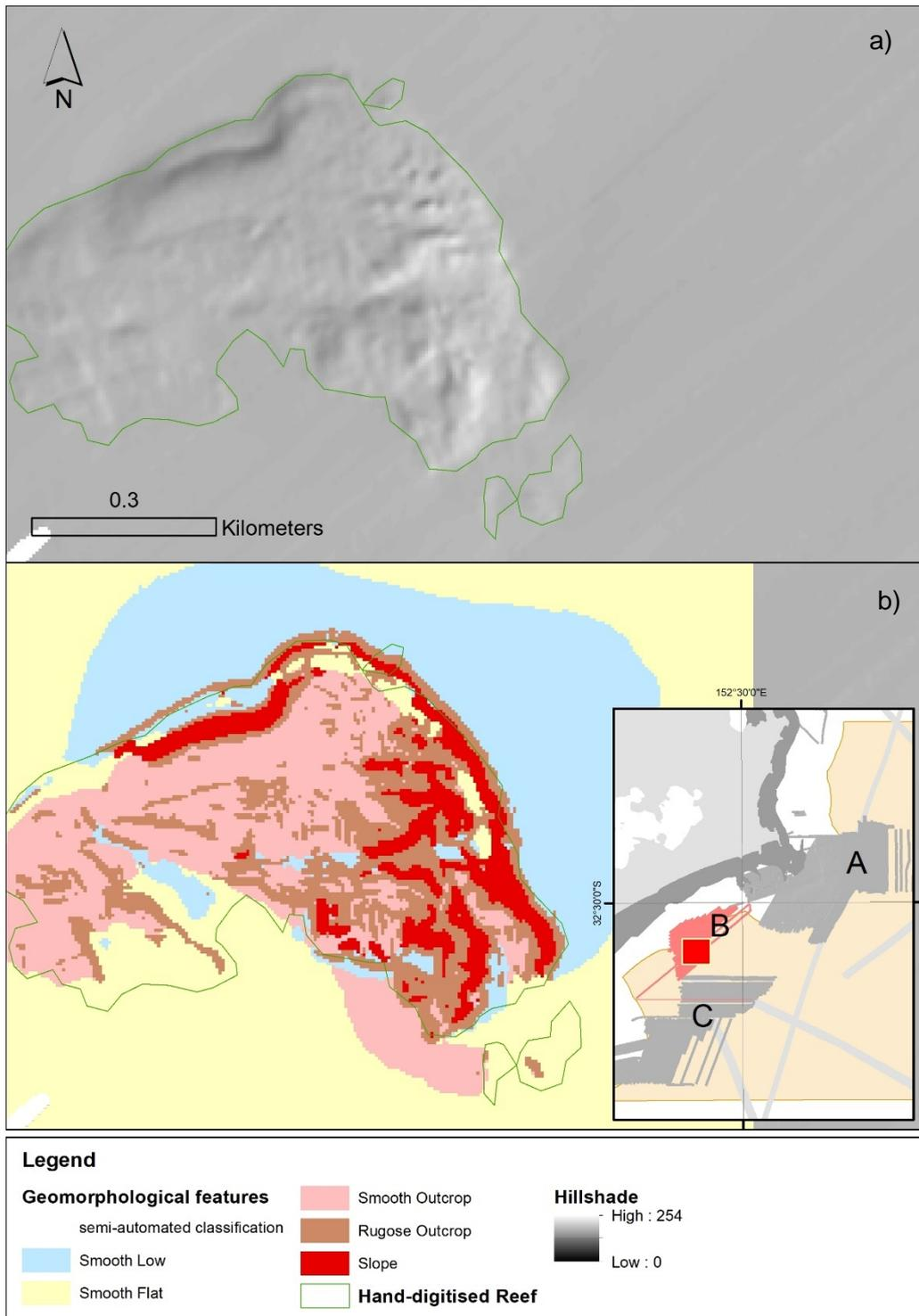
Figure 2-12. Sample area 1: a) hillshaded bathymetry showing relative relief, and b) shape file of colour coded geo-features; comparing hand-digitised (green polygons - supervised) and auto-classification (coloured polygons - semi-automated) techniques used for identifying seabed features in the Hunter Marine Park, at Outer Gibber (Area B).
