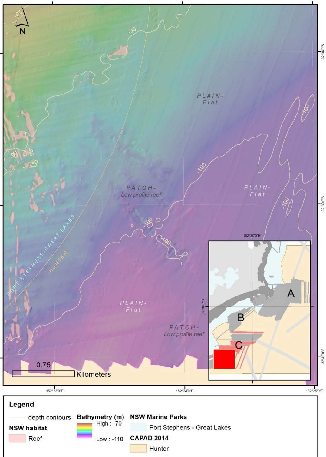
Figure 2-9. False-colour hill-shaded bathymetry of survey area C: Offshore Broughton and seabed features - southern section
