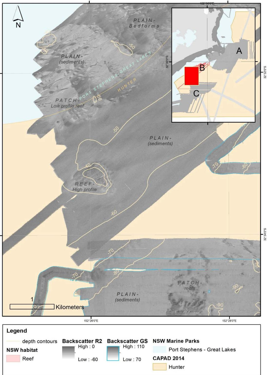
Figure 2-6. Greyscale backscatter (seabed reflectance) for survey area B: Outer Gibber & seabed features
