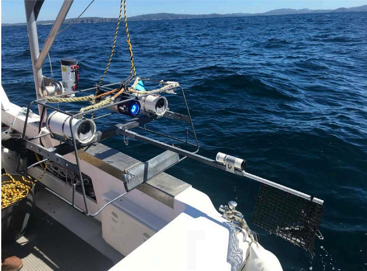
Figure 4-4. An example of a baited remote underwater stereo-video unit, including blue light, used in this study.
