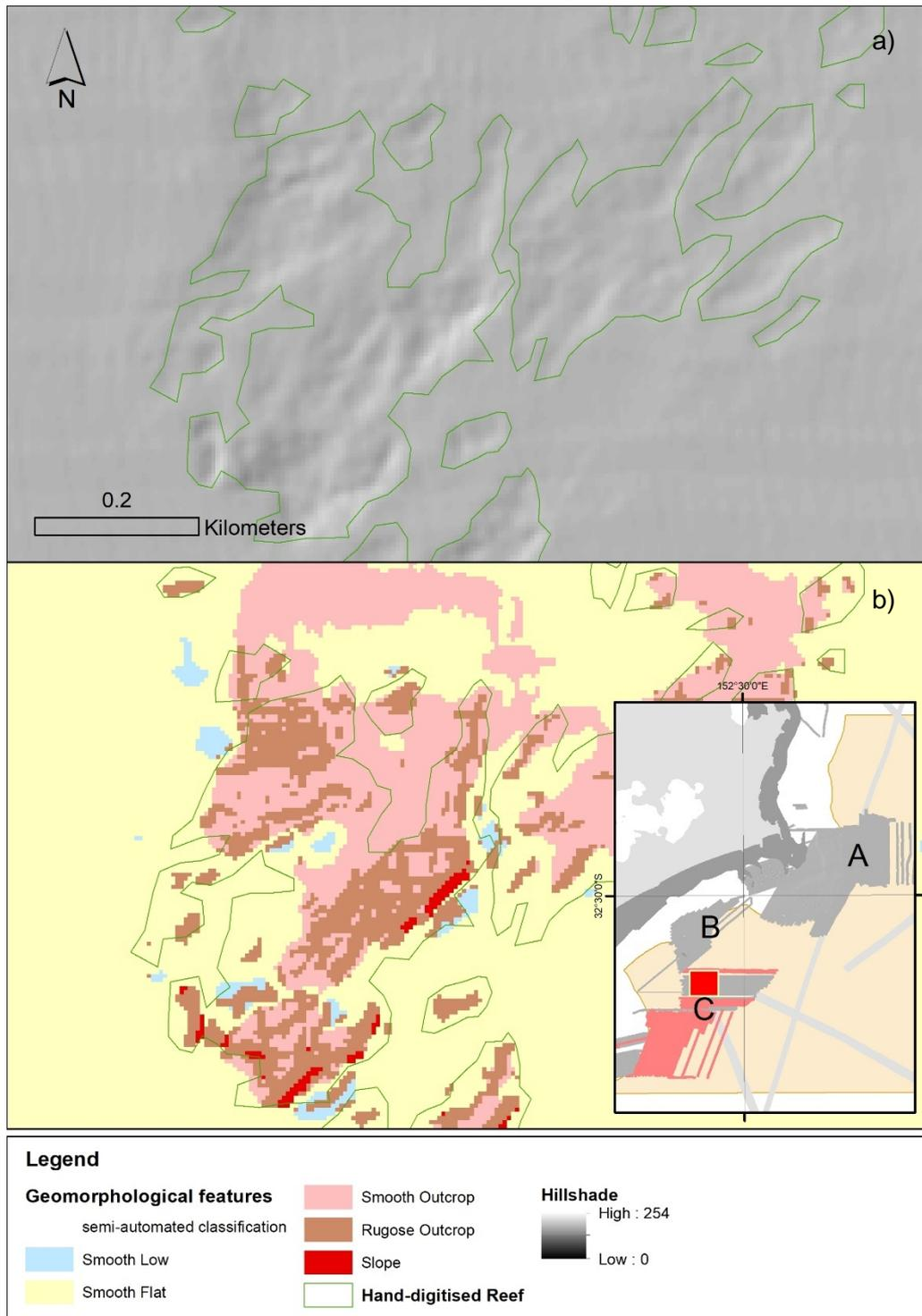
Figure 2-13. Sample area 2: a) hillshaded bathymetry showing relative relief, and b) shape file of colour coded geo-features; comparing hand-digitised (green polygons - supervised) and auto-classification (coloured polygons - comparing hand-digitised (supervised) & auto-classification (semi-automated) techniques used for identifying seabed features in the Hunter Marine Park, offshore of Broughton Island (Area C).
